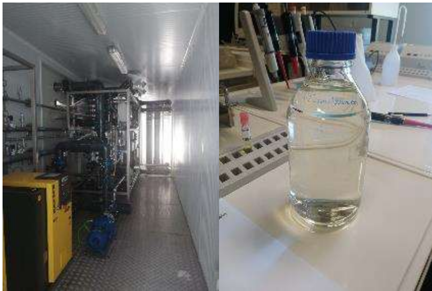
Figure 8 - Pictures of the ultrafiltration and chlorination unit and of the ultrafiltrated not chlorinated wastewater sample
